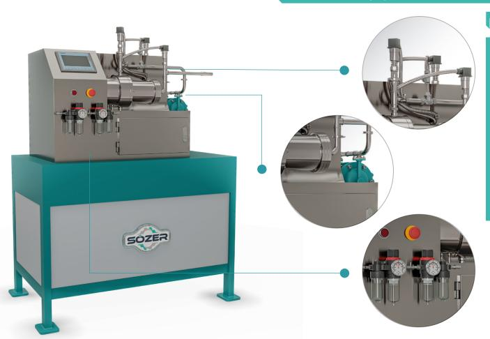
The usage area of nano horizontal milling machines begins in the applications where the wet milling of basket-mill machines is not sufficient. This type of machine, which can also mill in nano size, is widely used especially in continuous batch production model. It is a particularly preferred machine type for the production of nano-sized pigment milling and printing inks.
